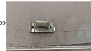
Align Left and Right Holes of Cover Plate Connector with Screw Holes
