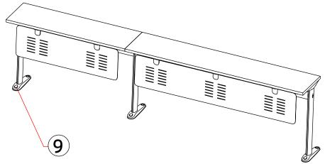
Supplier-provided screws for connecting to the ground: Self-tapping expansion screws
