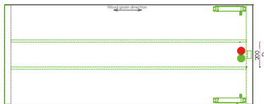
Socket Layout and Wiring Diagram for Double-Sided Independent Bar Counter
