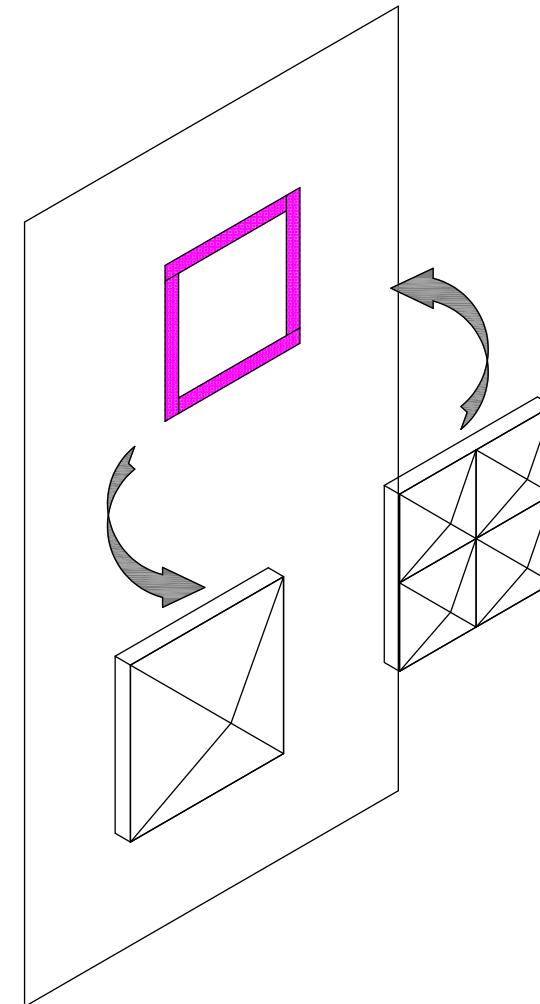
The Diamond is connected to the wall via a peelable adhesive. Therefore, it is not recommended to use this product on rough surfaces (such as unpainted concrete walls).
