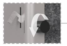
Lock Handle: Rotate the handle to the left to unlock and lock the latches that secure the two-sided writable whiteboard doors.
